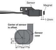
□ The center of the sensor is different from the center of the sensor case so be careful when mounting the sensor.
